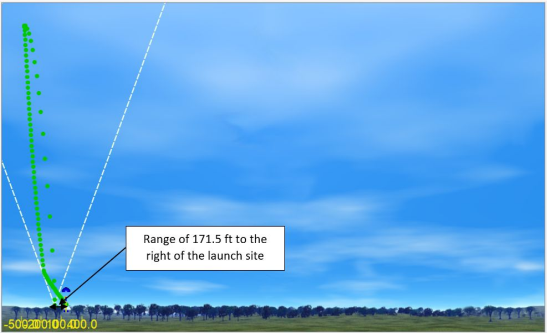
Figure 5.2-7 Range of Rocket After Launch at Light Wind Speeds
