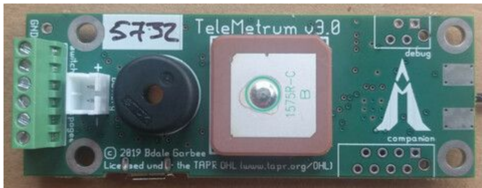
Figure 4.1.2.1-1 Telemetry v3 Top Image
